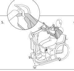
5. Standing. Maneuver the lift by pressing on the up and down buttons of the hand control (two speeds possible). The patient can actively participate by holding the crossbar and pulling himself/herself up.
